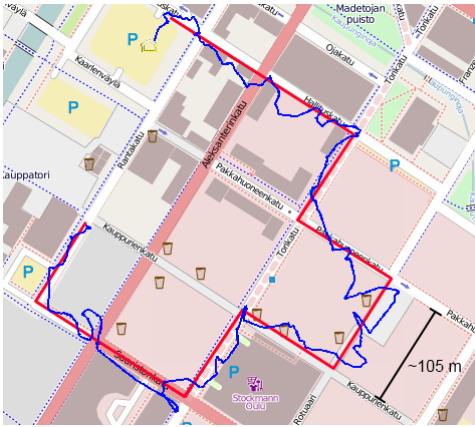
Figure 4. A typical GPS track. Red straight lines: the actual route. Blue zigzag pattern: the route recorded by the GPS.
